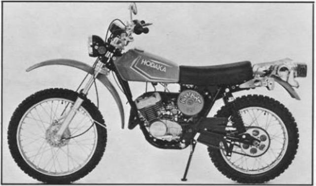
What you're looking at is the newest version of the legendary Wombat 125. It's street legal, dirt proficient. Rear shocks are gas/air, forks off the 250 give 7 1/4 inches of travel. Other trick goodies include folding shift lever, conical front hub, Preston Petty fenders, new tank design and \$675 price listing.
