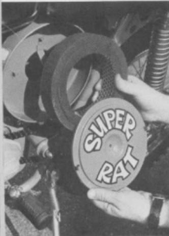
*The air cleaner is a dual stage washable foam element. Though very large, it required a lot of oil in thick dust.*
