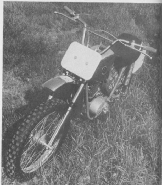
*The internal spring front forks work very well and have lots of travel. Large knobby tires provide good traction.*
